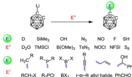
Scheme 1. Reactions between Lithiocarborane and Electrophiles (E + ) Yield C-Substituted Carboranes
